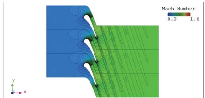
A flow passing through blade cascade was analyzed. Shock waves appear on blade surfaces. Analysis was performed for one entire blade and periodic boundary conditions were applied.
