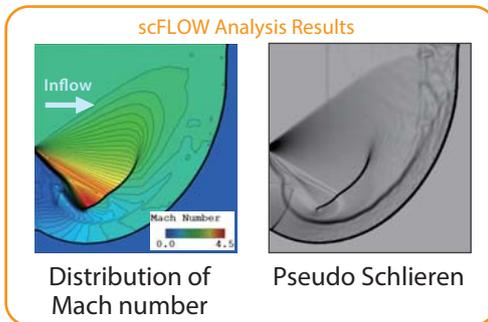
Diffraction of shock wave was analyzed. Shock wave comes from left side half up. Color shades visualized using pseudo Schlieren variable was in close agreement with Schlieren photograph on right. Overall, shock wave phenomenon was simulated accurately.
