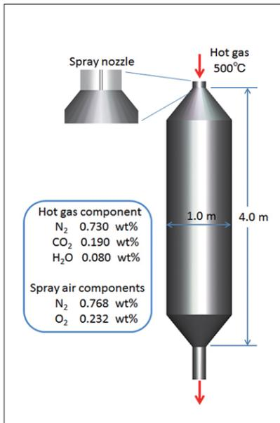
Figure 1: Spray air nozzle
