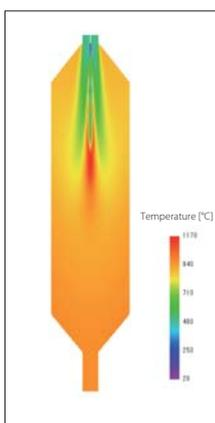
Figure 4: Behavior of fuel droplets and temperature distribution (8 sec.)
