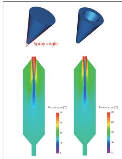
Figure 2: Temperature distribution (7 sec.) Full-cone (left), hollow-cone (right)
