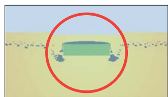
Figure 5: Water percolation to sand (with resin installed)
