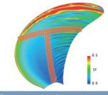
Changes in streamline positions and increasing wall friction coefficient along the blade surface, due to boundary layer turbulent transition, agreed with experiment
