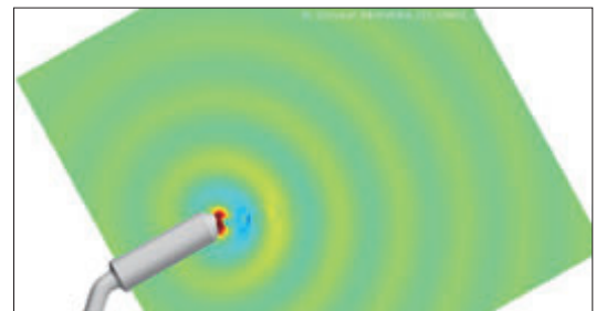
Sound pressure distribution inside/outside an exhaust pipe (when noise source is used with M=0.2)
