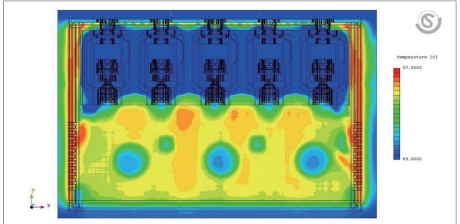
Figure 4: Air temperature distribution field (longitudinal section)
