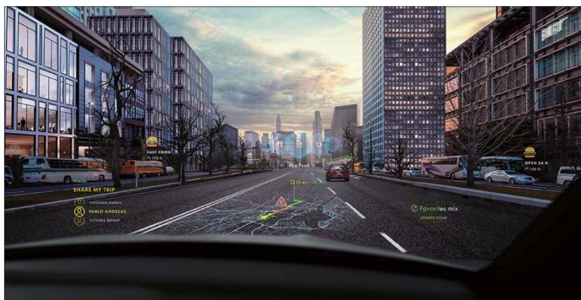
Figure 1: Virtual image projected through the windshield on the road
