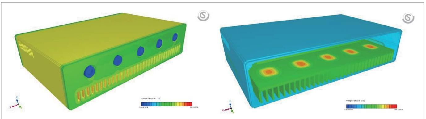
Figure 3: Temperature distribution fields of laser unit components
