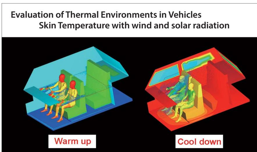
Figure 2. Evaluation of thermal environments in vehicles Skin temperature with wind and solar radiation. Simulated using SC/Tetra version 7.
