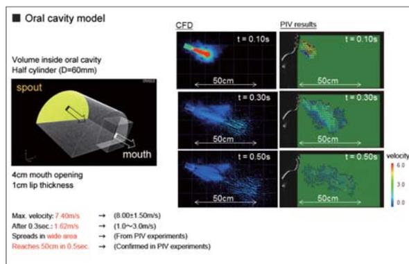
Figure 1. Development of a model for airflow of coughing with a modeled oral cavity
