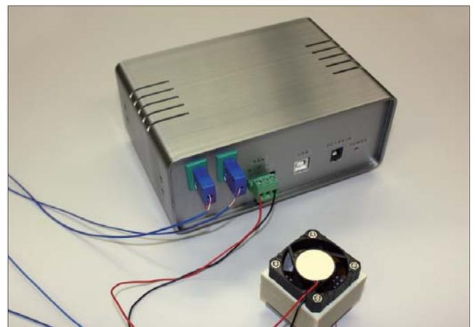
Fig. 2 Heat generation amount measurement system
