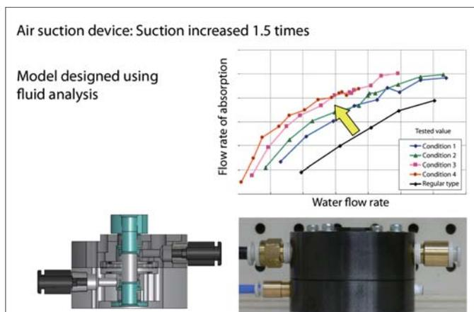
Figure 3: Designing an air suction device with 1.5 times greater suction, without producing prototype
