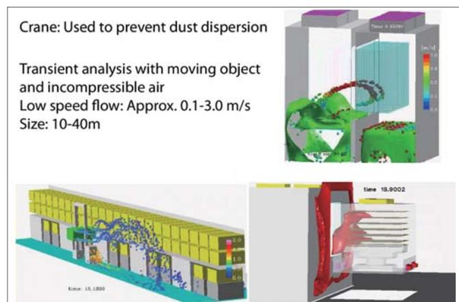
Figure 4: Simulation of clean room crane and dust dispersion. Using overset grids and moving object, transient analysis with incompressible air and low speed flow (approx. 0.1-3.0 m/s) was undertaken in 10-40 meter size.
