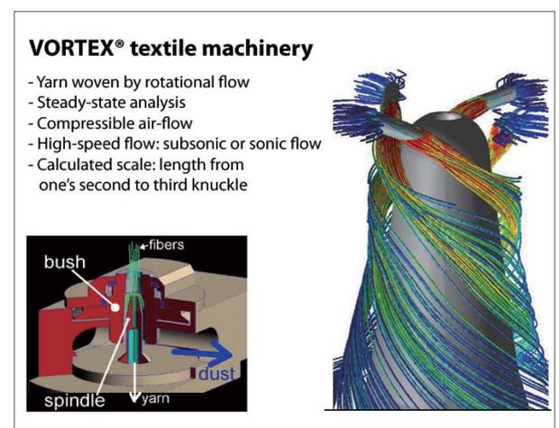
Figure 2: Application example of SC/Tetra for development of VORTEX® third generation. Steady-state analysis was undertaken to evaluate compressible air-flow in the space where yarn is woven by rotational flow.
