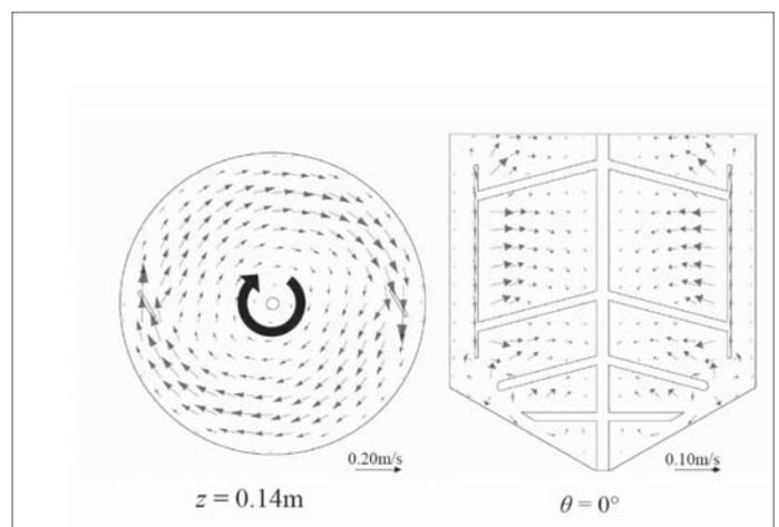
Figure 3: Velocity vector distributions of r-θ plane and r-z plane (Impeller 1 Normal rotation)
