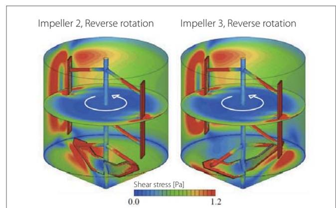
Figure 6: Shear stress distributions of the wall surfaces and r-θ planes (Impeller 2 and Impeller 3)
