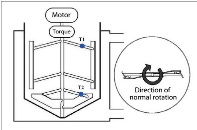
Figure 1: Schematic diagram of experimental equipment (Impeller 1)
