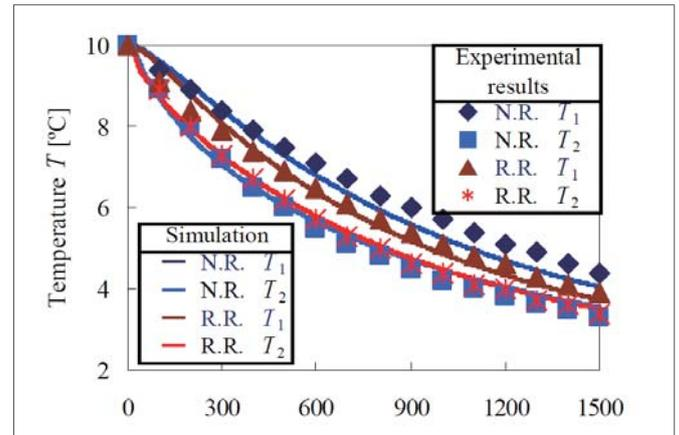
Figure 2: Comparison of rotational directions for Impeller 1 (Plot: Experimental result, Line: CFD result, Normal rotation: N.R., Reverse rotation: R.R.)
