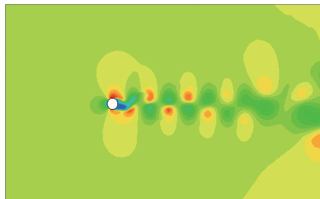
Figure 1: Analysis of unsteady laminar flow around a cylinder to understand a unsteady flow field
