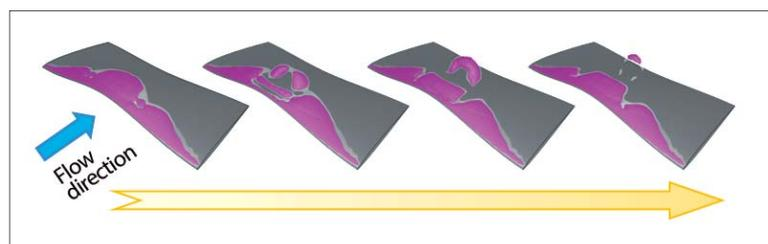
Fig 1 Predicting the occurrence of transient cavitation around the three-dimensionally twisted turbine under water (red area indicates the predicted cavitation)
