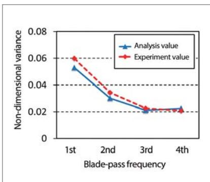
Fig 6 Pressure fluctuation on the surface of the ship
