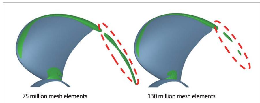
Fig 7 Predicting cavitation occurring within the eddy near the turbine edge
