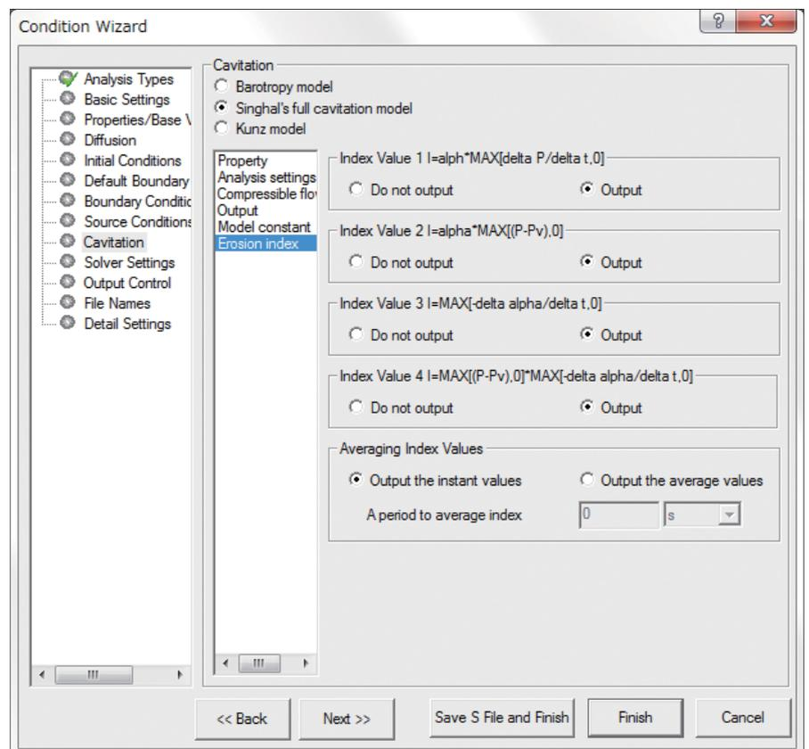
Fig 3 Output setting window of simplified index
