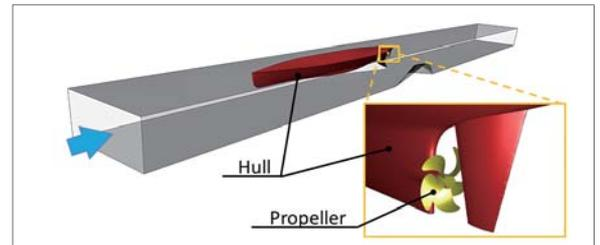
Fig 4 Analysis model of marine propeller
