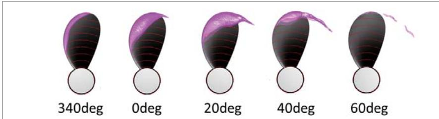
Fig 5 Predicting the occurrence of transient cavitation on propeller turbine surfaces
