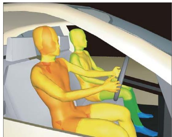
Figure 1: Analysis of SC/Tetra coupled with JOS function to predict the temperature changes of the passengers in a vehicle
