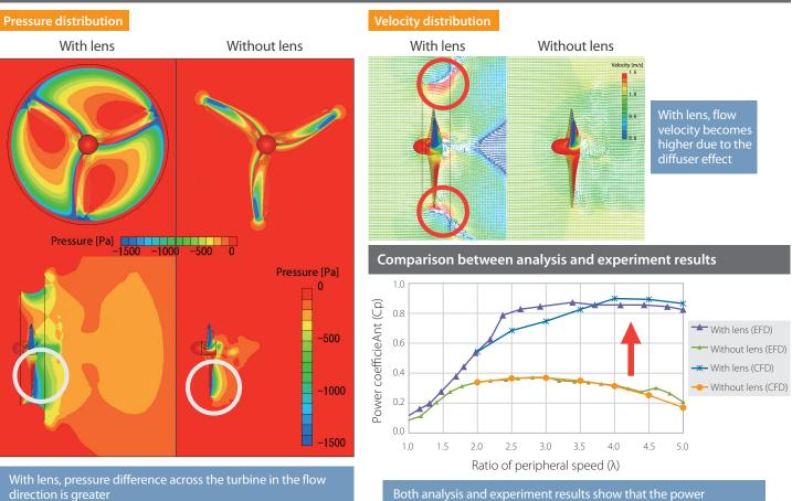
Both analysis and experiment results show that the power coefficients increase by more than double when the lens is attached
