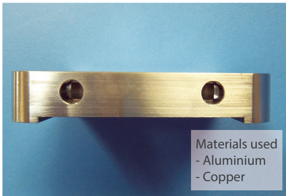
Cross section of a water-cooled plate
