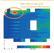
Index for age of air is high in one area, meaning ventilation effectiveness is low. This is caused by circling air flowing from outside through the nearby opening and from the closest blower.
