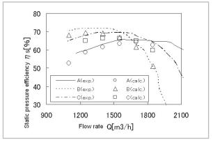
Maximum Static Pressure Efficiency (B) > (C) > (A) Air Capacity at Best Efficiency Point (A) > (C) > (B)
