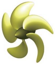
**High skew propeller of Seiunmaru**
