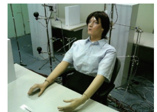
Experiment using thermal mannequin
