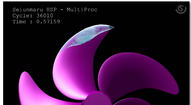
Cavitation generated around screw propeller (Volume rendered by bubble radius)
