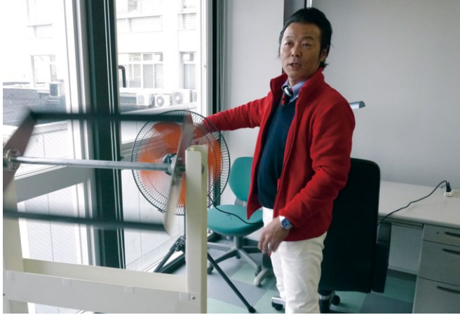
Picture 2: Demonstration of wind minimizing device Strong wind changes to a gentle breeze as the device rotates
