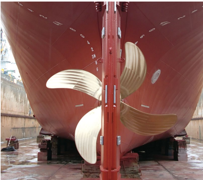
Picture 2: Propeller for chemical tanker Unique stripe patterns on Nakashima Propeller products, the Nakashima-Patterns, are known as their signatures
