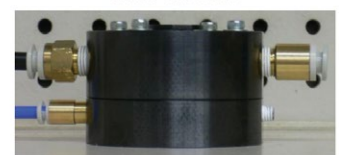
Figure 3: Designing an air suction device with 1.5 times greater suction, without producing prototype
