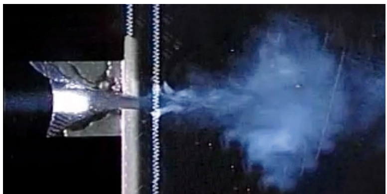
Fig. 2: Smoke-wire flow visualization of a synthetic jet
