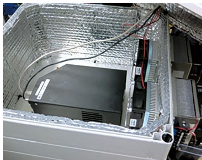
Picture 2: Inside of spectroscope of hair inspection unit
