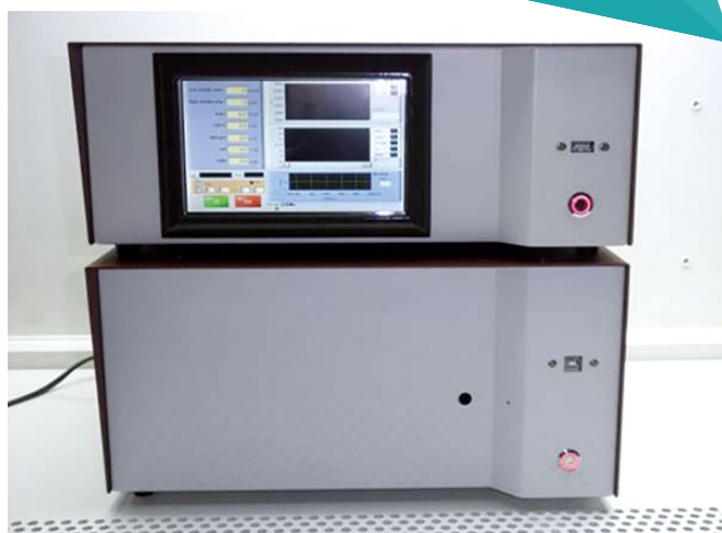
Picture 4: Heat generation of wood pellet and moisture inspection device Control unit (above) and chassis for spectroscope (below)
