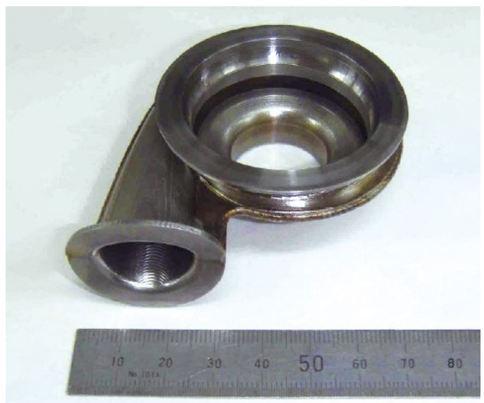
Fig. 6: Turbocharger improvement — The turbine scroll was made thinner and wrapped with heat insulator in an effort to increase turbine power.
