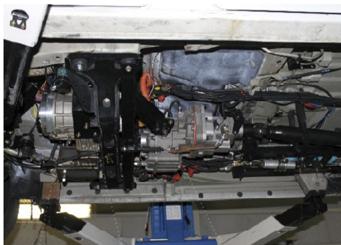
Drive motor Diesel engine Power generator
