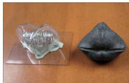
Figure 1: A model and fossil of a brachiopod (spiral thin bones are reproduced by aluminum wires for water flow tests)
